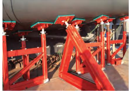
Wooden blocks and packers are always positioned between the cradle supports and the hull / keel. Cradle "wedges" are secured to the deck with ISO regulated corner castings. All other cradle structures are welded to the deck and to spread the load efficiently soft wood keel blocks will be added at every frame interval.
